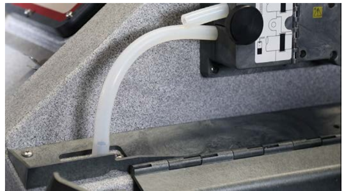
Figure 6. Pump tubing connected to the bulkhead fitting at exterior (shown: 5800).
