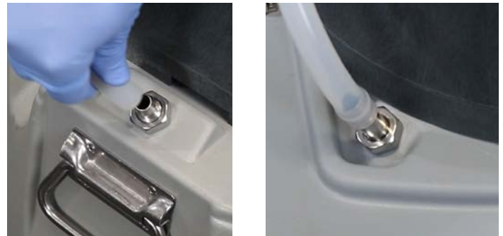
Figure 5. Connecting pump tubing to the bulkhead fitting (shown: 6712 (left) and BLZZRD (right)).
