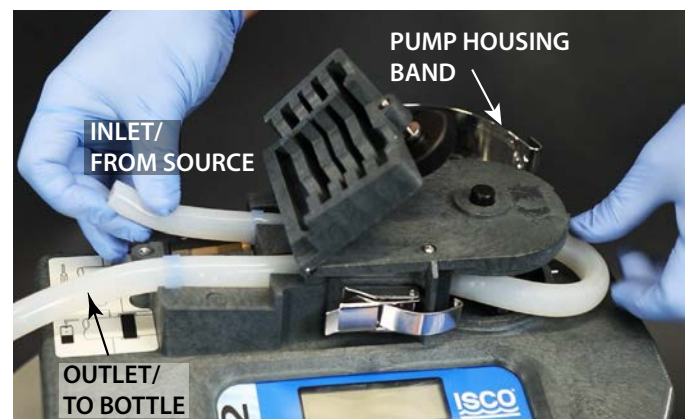
Figure 1. Removing and replacing the pump tube (shown: 6712; BLZZRD is similar).
