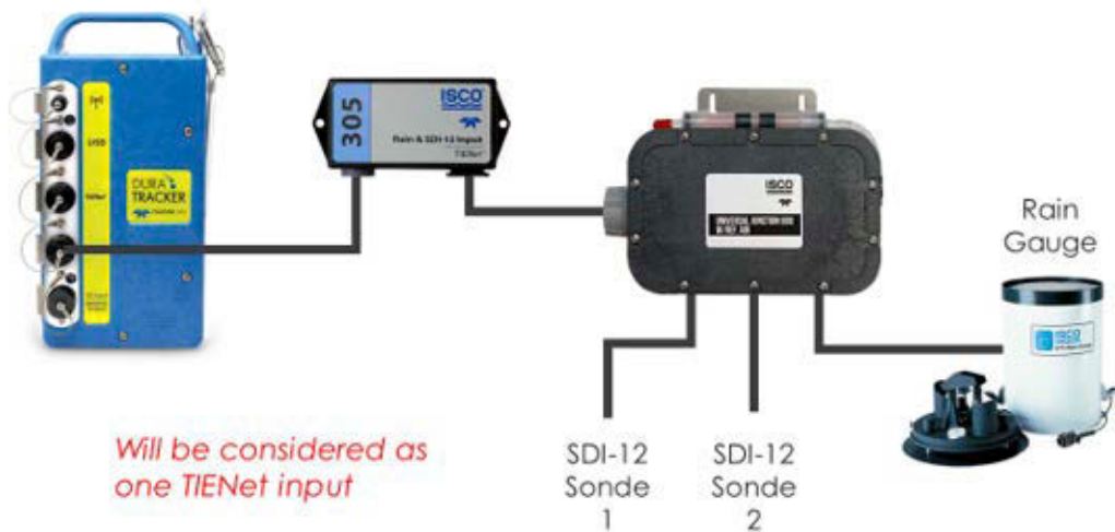
Figure 1-3 TIENet connection to Rain Gauge and SDI-12 Sonde via the 305 Rain & SDI-12 Input
